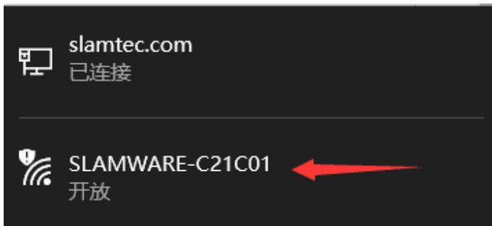
Please connect to the SLAMWARE-XXXXXX via WiFi(you can also connect the SDP Mini to your PC via network cable, in this condition, the network adapter on the PC should be set as DHCP mode). Then open the tool *Robot Studio* in the *bin* folder of the SDK downloaded above and use the default IP address *192.168.11.1* to connect to the SDP Mini, if successfully. The scanned map will show up in the Robot Studio interface.
