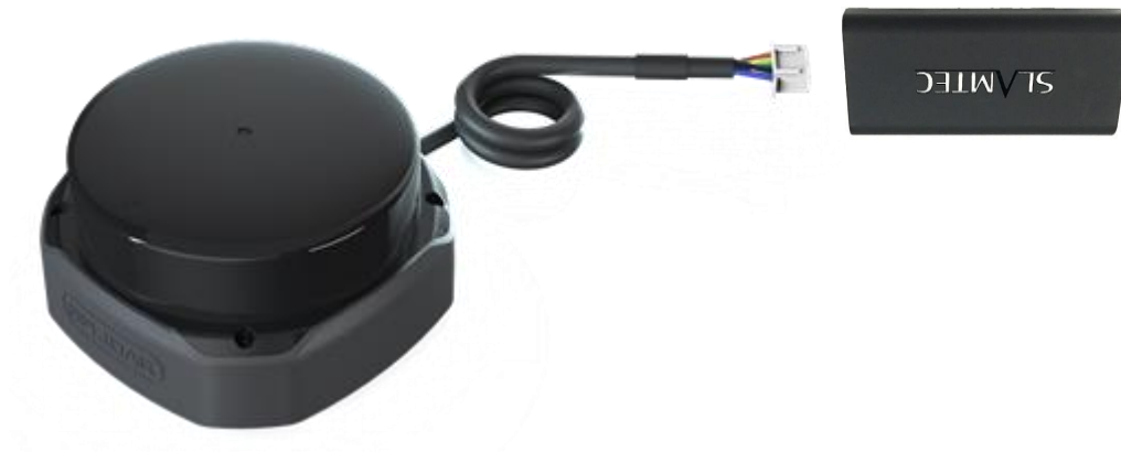
Figure 2-1 Connect RPLIDAR S2 and USB Adapter
