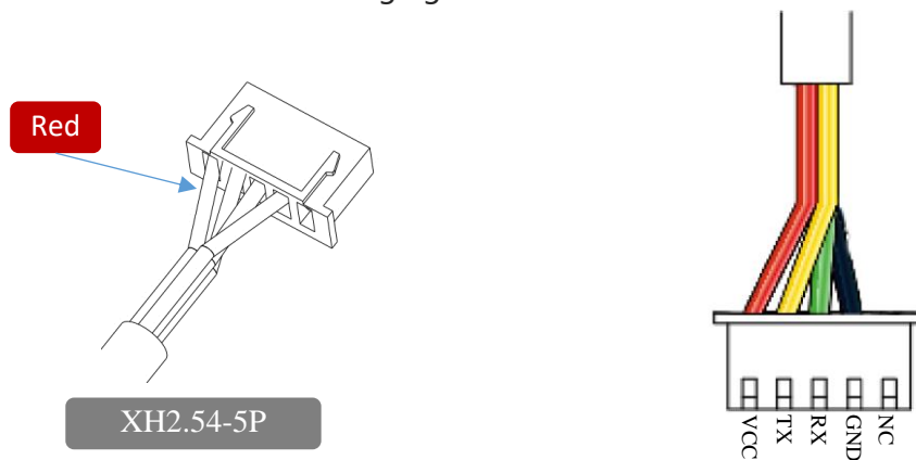
Figure 2-5 RPLIDAR Power Interface Definition
