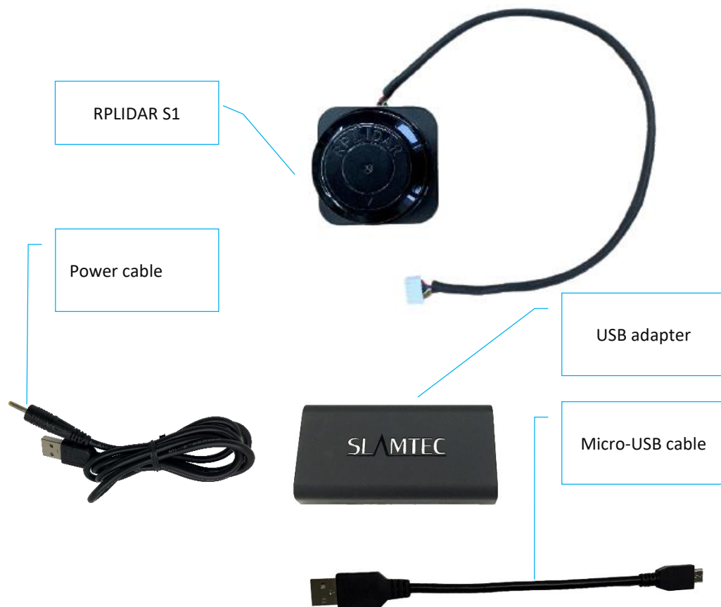
Figure 1-1 Items in the RPLIDAR Development Kit
