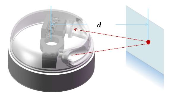
Figure 1-2 The RPLIDAR Working Schematic
