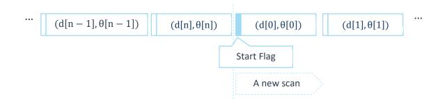
Figure 1-5 The RPLIDAR Sample Point Data Frames
