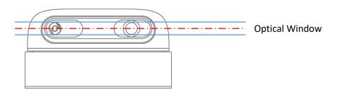
Figure 2-3 RPLIDAR Optical Window
