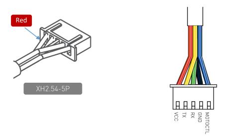
Figure 2-5 RPLIDAR Power Interface Definition
