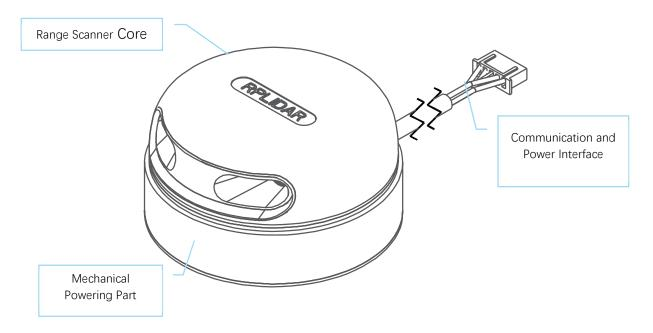
Figure 1-1 RPLIDAR System Composition
