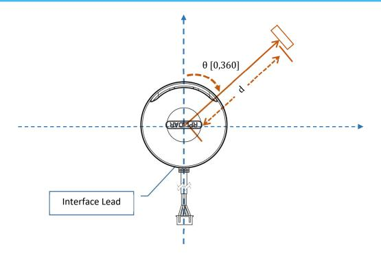
Figure 2-4 RPLIDAR Scanning Data Coordinate System Definition
